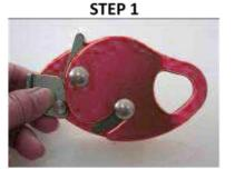
Hold the Rope Grab in the correct up-and-down direction
