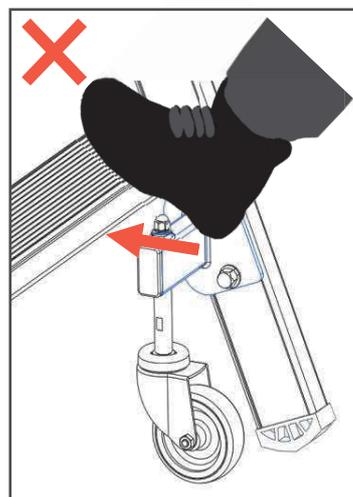
When accessing the platform, put you feet vertically on the first step so the platform doesn't move and the platform uprights touch the ground.
