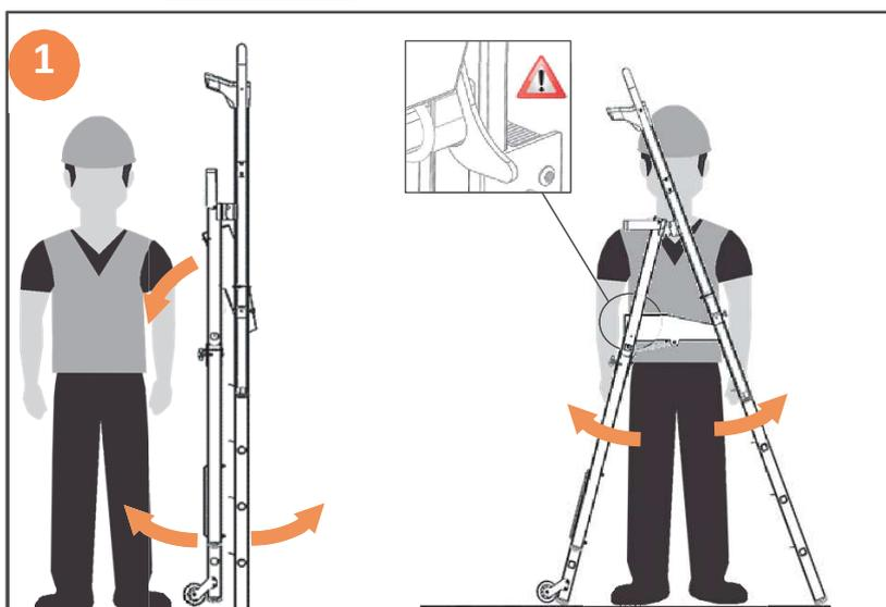
Hold the product vertically to unfasten the security belt, then, taking stiles, open platform by discarding ascendable side from support side. Check that the platform is in contact with the support side and that platform lock is engaged.
